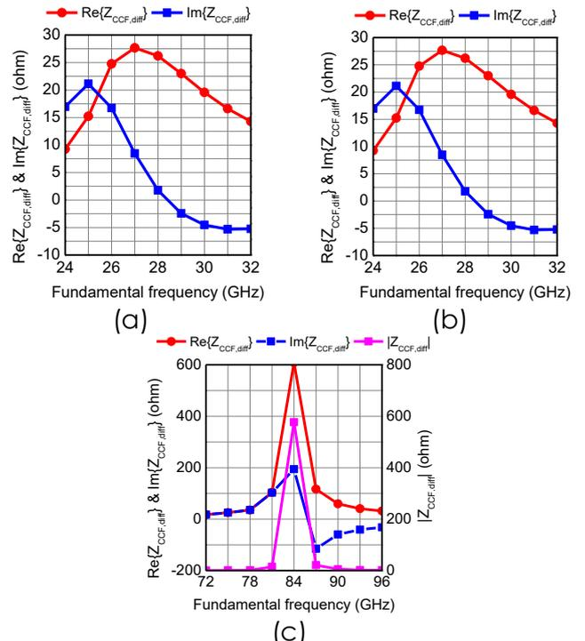
Fig. 3. Frequency response of  $Re\{Z_{CCF}\}$ ,  $Im\{Z_{CCF}\}$ , and  $|Z_{CCF}|$  at (a)  $f_0$ , (b)  $2f_0$ , and (c)  $3f_0$ .
