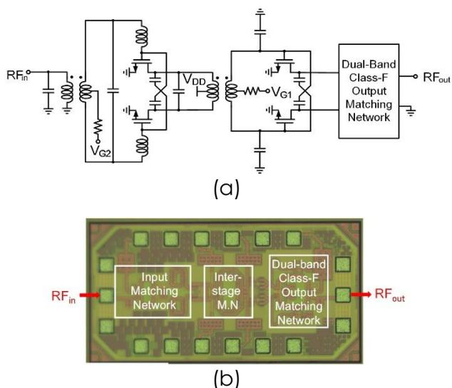
Fig. 5. (a) Schematic, and (b) chip photo of the dual-band class-F PA.
