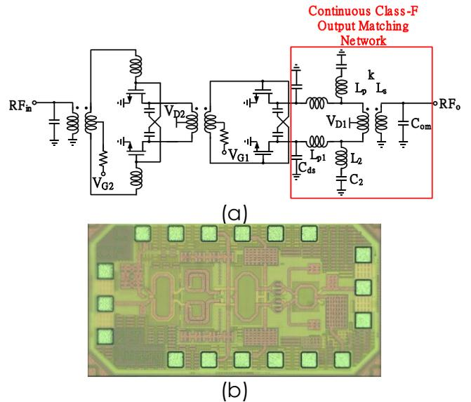
Fig. 1. (a) Schematic, and (b) chip photo of the CMOS CCF PA.
