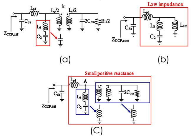
Fig. 2 Equivalent half circuits of proposed CCF output matching network at (a)  $f_0$ , (b)  $2f_0$ , and (c)  $3f_0$ .
