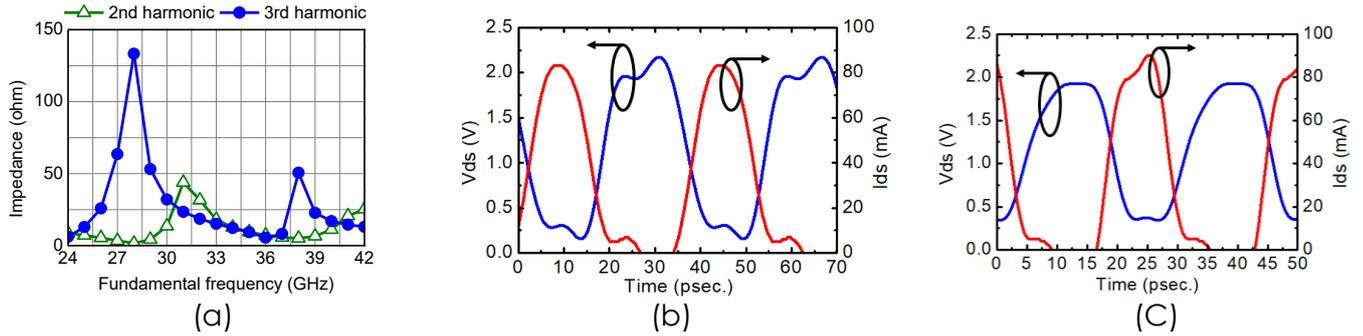
Fig. 7. (a) Simulated harmonic impedance of the proposed dual-band class-F output network, and simulated drain voltage and current waveforms of output transistor at (a) 28 GHz with  $P_{in} = -2$  dBm and (b) 38 GHz with  $P_{in} = 0$  dBm.
