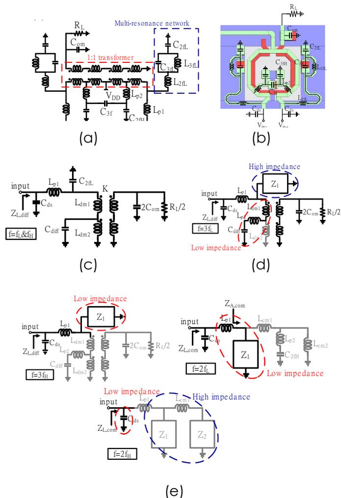
Fig. 6. (a) Detail schematic, (b) layout of the proposed dual-band output matching network, and its equivalent circuits at (c) fundamental, (d)  $3f_L$ , (e)  $3f_H$ , (f)  $2f_L$ , (g)  $2f_H$ .
