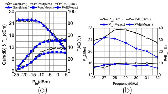
Fig. 4. (a) Gain, output power, and PAE versus  $P_{in}$  at 27GHz, and (b)  $P_{sat}$  and peak PAE versus frequency.
