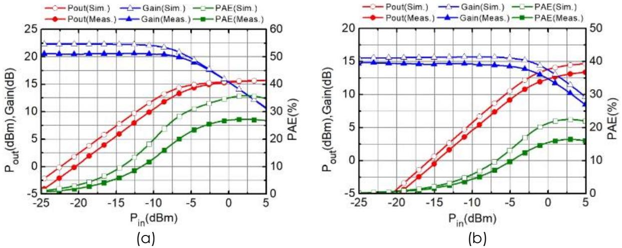
Fig. 8. Large-signal performance versus  $P_{in}$  at (a) 28GHz, and (b) 38 GHz.
